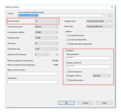
Make sure the 'Archive format' is set to 7z and leave the 'Encryption method' at AES-256. Once you have given an appropriate name to the zip file, you can enter a password. If you also want to make the names of the files in the zip file unreadable, select 'Encrypt file names'. This is only recommended if the file names themselves contain confidential information. Press 'OK' and the encrypted file will be created.
