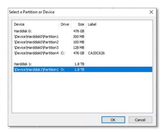
Select the encrypted disk and press 'OK'. You have now selected your encrypted drive and the letter you want to mount it to. Then press 'Mount'. Because the disk is encrypted, you will be asked to enter the password.
