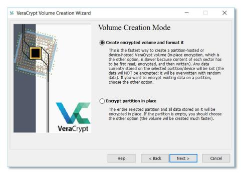
If you want to save and encrypt the data that is already on the disk, you need to select the second option ('Encrypt partition in place'). Because here the process does not start with a blank disk, choosing this option will take longer.
