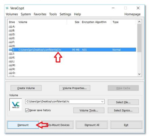
Proceed as follows: first select the disk you want to unmount in VeraCrypt and then press 'Dismount'. Then the virtual disk will be unmounted and disappear from your system. The file container is now encrypted and what remains is the (unreadable) encrypted file you started with in step 1.
